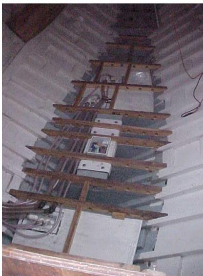
The three tanks he made were then put in place and the water and vent lines were run. The forward smaller tank, we have discovered, has the water, vent line backwards, and needs to be fixed. Luckily, this can easily be resolved by lifting one of the cabin sole hatches and using a few hose clamps. Once completed, this will give us 73.5 gals. of fresh water in out tanks. Skip will put in a reverse osmosis system as well; this will allow us to turn salt water into fresh water at one gallon an hour.
