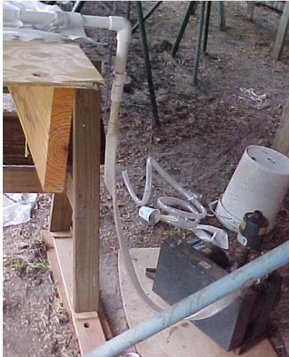
Vacuum bagging the cabin side. The sides are 3 layers of  $\frac{1}{4}$ " Euro-lite plywood, cold-molded over a form. By vacuum bagging, Skip achieved approximately 1800 lbs. per sq. ft. of clamping pressure.
