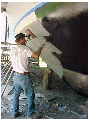
That evening in just a few hours, Skip put on a heavy layer of coal tar epoxy under the waterline. This coating would give MISTRESS a great water barrier and would fill any pinholes in the primer.
