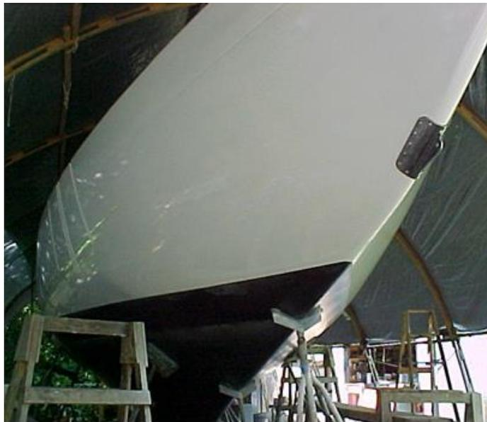
By the end of May 2004, Skip has sprayed two coats of Fleet White Awlgrip onto MISTRESS's port side. I find it impossible to shoot pictures because of the mirror images, which reflect in the hull, the dog pool, the frames to the building, even the grass.
