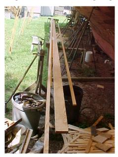
He made from yellow pine her new starboard 46' sheer clamp and shelf. It started as a 24' long,  $2 \times 12$ . Her ripped it into two 24' -  $2 \times 6$ 's. Then he scarfed it together to make a 46'  $2 \times 6$ . It would be fastened into place with lots of clamps and bolts.
