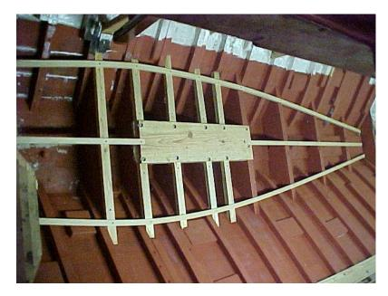
You can also see the interior is gone, which made it rather precarious for Skip to work on until he put down a temporary cabin sole. All tools, fasteners, and even the Shipwright constantly slide into the bilge.
