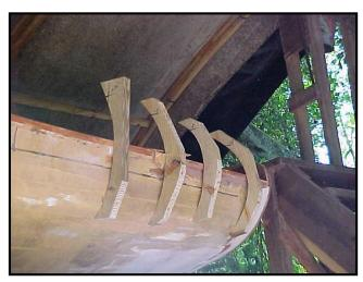
Starting with the 6" radius on the transom the temporary molds were cut to shape for the bulwarks.
