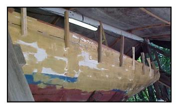
Using scrap wood Skip made these strips and fastened them to MISTRESS. The inside shape is the shape he wants the bulwarks to end up with. When I ask him how he figures these things out, he simply says, "I know what I want for the final shape and then I just work backwards". I realize this is much easier for him to see than someone like, myself. I believe it must be the artist in him who so easily sees what the end-product will look like.
