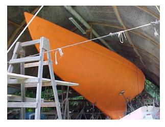
This picture shows MISTRESS pretending to be the big giant pumpkin. With her second coat of red lead, the transom glassed over, the keel faired in, and the chain plate impressions set in, she is now a fully restored wooden boat hull and is ready for glassing.
