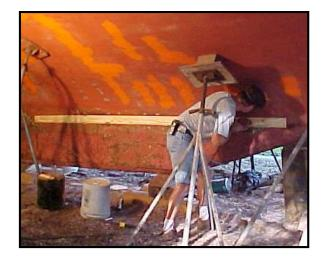
In this photo, Skip is fairing in the keel. She was originally fitted with stone ballast, however, sometime in her past it was removed and iron was attached to compensate for the weight. You can also see the first coat of red lead has been painted on her hull.
