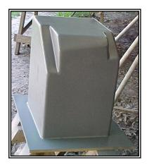
This is the template. He has put the wood pieces together and faired it. He will then fiberglass the outside. This should allow just enough space for a propane tank and the fittings necessary for the lines that will carry the propane to the stove. It will also be watertight.
