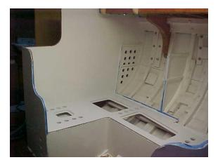
The locker with the small opening is where a new 20-gallon water tank will go which we will purchase instead of the ones Skip made housed under the cabin sole. Outboard there are three, though you can only see two in this photo, lockers that will hold can good storage. Not yet in place will be three additional lockers behind the seat cushions. One locker is for Skip's stuff, one for food storage, and one is for the water maker.
