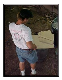
Skip begins work on the propane tank lockers. There will be two, one on either side of the cockpit set flush with the deck. He will spend 40 hours building the template for this project and then lay up the final product in fiberglass. One locker will have lines running to the stove the other is for stowage of a spare tank. Each locker will hold a 20 lb. tank. In this picture, we see parts for the template, odd shaped pieces that will somehow come together to make the outer shape of the locker.
