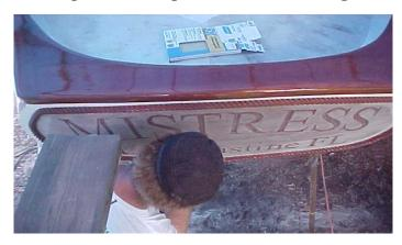
...six layers of Bristol Finish are put on in one day. After two years, that Bristol still looked good. Here, after bleaching, staining and five coats of CPS he put 12 coats of epiphanies and 5 coats of Albright. This does not include the gold he would use on the carved rope and lettering.
