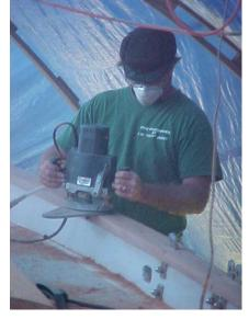
Here Skip is routing the cap rail to shape. He will then sand it all to 220.
