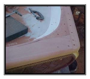
This week Skip is working on the caprail, made from 1 &  $3/8^{th}$  inch thick mahogany. He joined the rail with shiplap scarf joints and teak butterflies. There is a  $\frac{1}{4}$ " deep groove in the bottom of the cap rails, which fits over the top of the bulwarks. The cap rails are bedded in polysulfide and screwed every 8" with 3 &  $\frac{1}{2}$ " #14 SS screws. Skip says it took him 40 hours to get this done.
