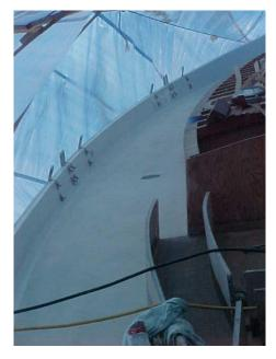
We left off last week looking aft. This view is port side looking forward and shows one of the prisms in the side deck. There are six in all and often allow enough light for reading, and on a bright day, it's like looking at a 100-watt light bulb. In the evening, each prism lights the way utilizing either the red or, white lights, from below. There is one is in the saloon, one over the chart table, one in the galley, one in my office, and one forward of the forward chain locker.
