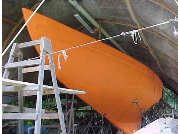
This picture shows MISTRESS pretending to be the big giant pumpkin. With her second coat of red lead, the transom glassed over, the keel faired in, and the chain plate impressions set in, she is now a fully restored wooden boat hull and is ready for glassing.
