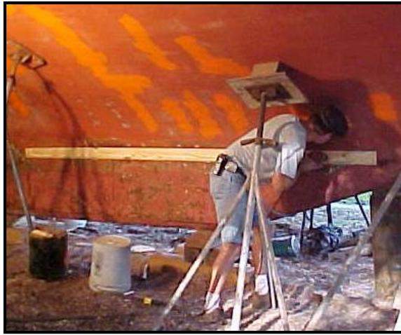
In this photo, Skip is fairing in the keel. She was originally fitted with stone ballast, however, sometime in her past it was removed and iron was attached to compensate for the weight. You can also see the first coat of red lead has been painted on her hull.
