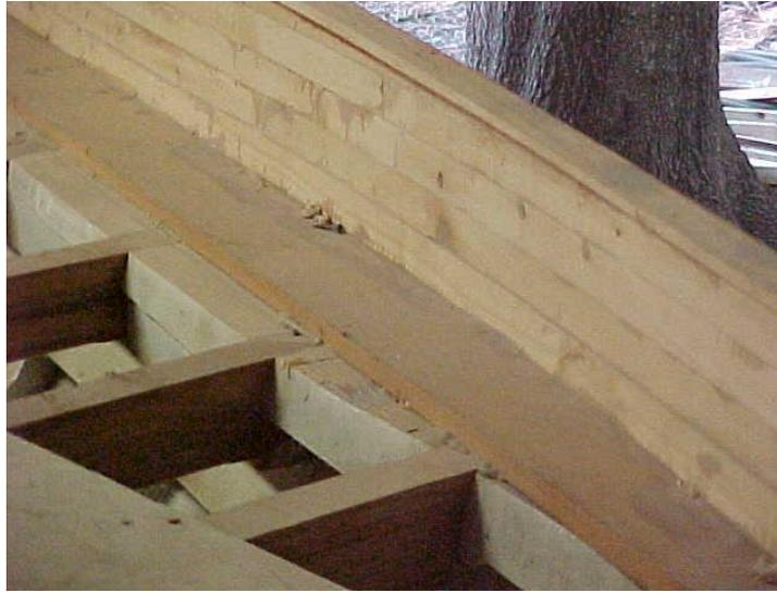
The first strip went down on the deck, clamped tight to the temporary molds, then fastened to the deck. Each layer he then built upon the one before as he fastened it all with glue and 3 & 1/2" nails, every 6 inches.
